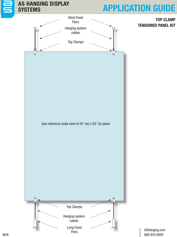
This assortment includes Short Fixed Piers (2x), stainless steel upper-system cables (2x), Top Clamp (4x), stainless steel lower-system cables (2x), Long Fixed Piers (2x), and attachment hardware and other fittings. Assortments are available in each of three Top Clamp sizes. Display panels are not included.
