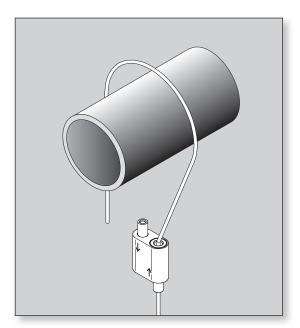
Loop a steel cable over the supporting element and back to the hanger.
