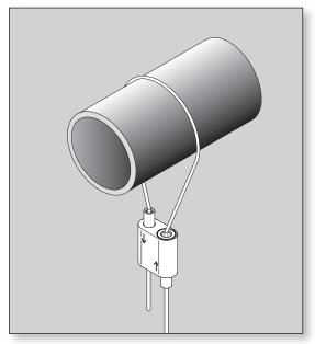
Complete by passing the cable through the second cable gripper, again in the direction of the arrows.
