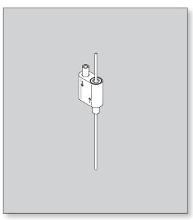
Insert the cable as shown by the arrows.
