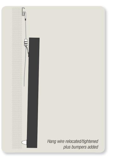
Where to locate the attachments? That depends on the size and weight of the frame. The rule of thumb is that you want to mount these as high as possible on the frame side rails, but just low enough so that the system hook will still be hidden behind the frame top. When you support the frame from your finger at the center of the hang wire, the wire should be no closer than 1-1/4" – 1-1/2" from the frame top edge.
