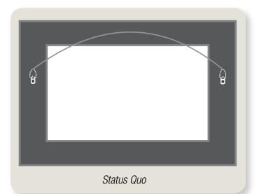
**ACTION:** Simply move the "hang wire" attachment points upward on the frame and while doing so, remove the extra hang wire length.
