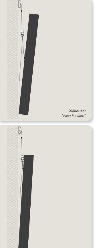
Hang wire relocated and tightened
